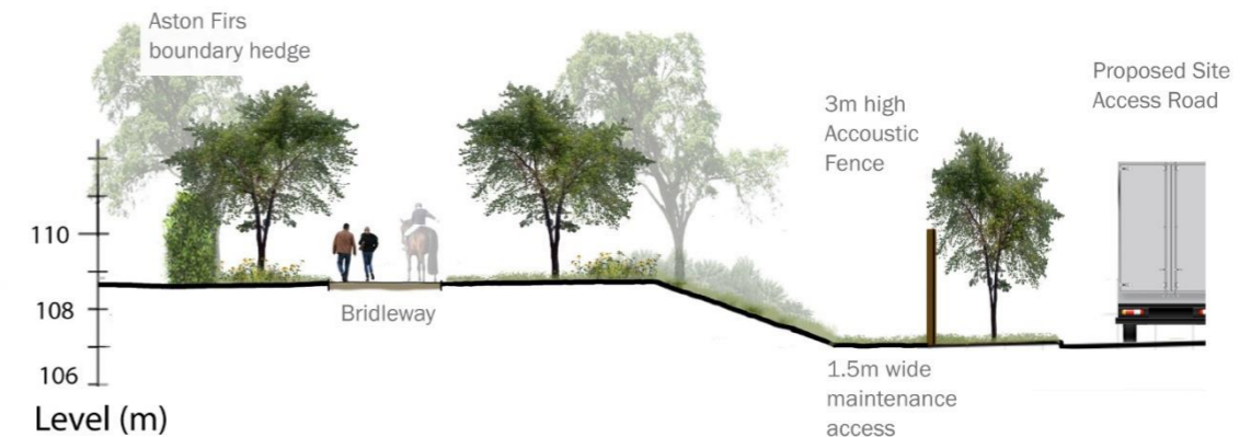
Fig 64. Section D-D – Close Boarded Timber Panel Acoustic Fence Proposal.
